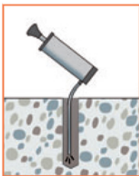
Clean hole (blowing)
