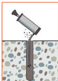
Clean hole (blowing)
